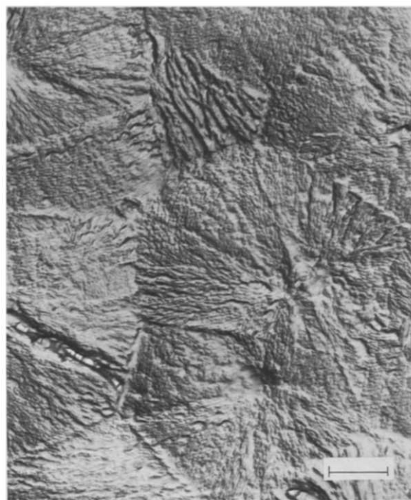
Figure 6 Spherulitic textures of the PEO mixture crystallized via the same three-step procedure as used in Figures 2 , 3 and 4 . The scale bar is 0.5 \mu\text{m}
