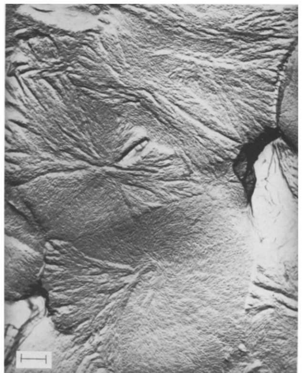
Figure 3 Spherulitic textures of the PEO mixture crystallized via the same three-step procedure used in Figure 2. The scale bar is 0.5 \mu m
